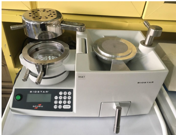
Figure 1-A: A vacuum forming machine for which the heating element is acting on the vacuum-formed retainers.
