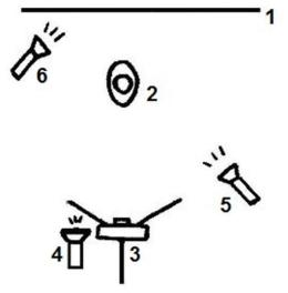
**Figure 1:** A Photographic set up (1. background, 2. subject, 3. camera with tripod, 4. primary flash, 5. secondary flash, 6. projector)
